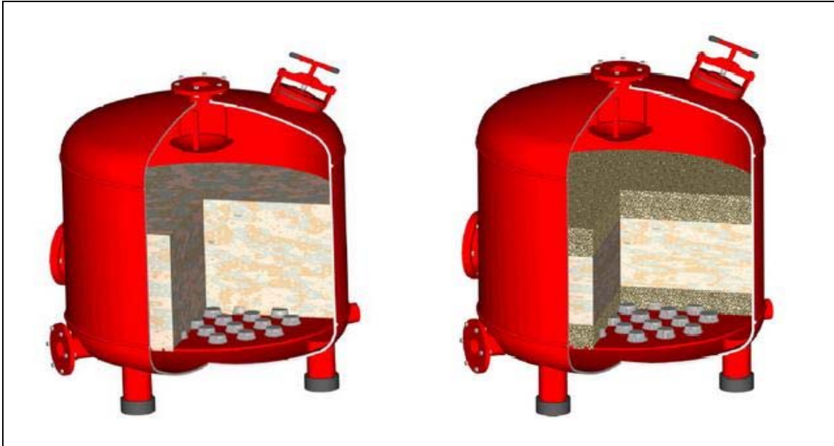
Figure 3. Basic scheme of a monolayer and multilayer filter. http://galeon.com
